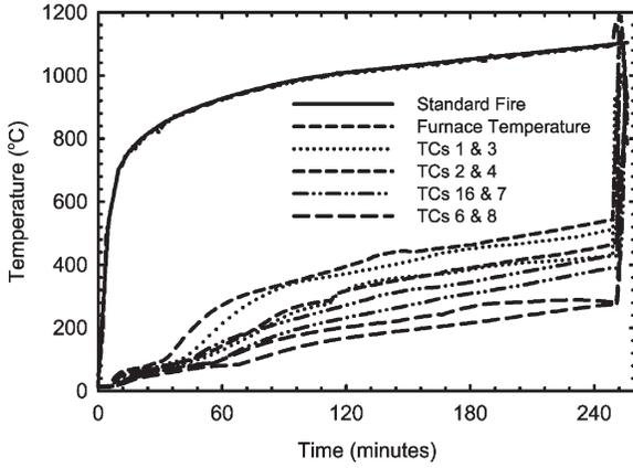
Fig. 5—Temperatures recorded at various locations in Column SQ2 as a function of fire exposure time
