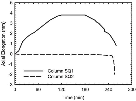
Fig. 6—Comparison of axial deformations as a function of time for Columns SQ1 and SQ2
