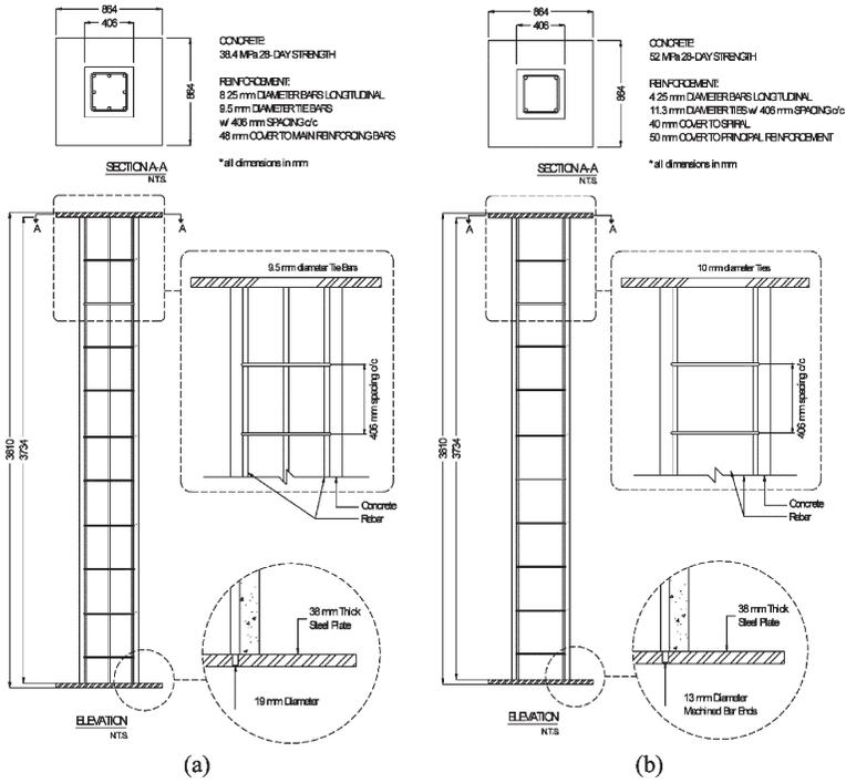
Fig. 1—Elevations and cross sections for Columns SQ1 and SQ2
